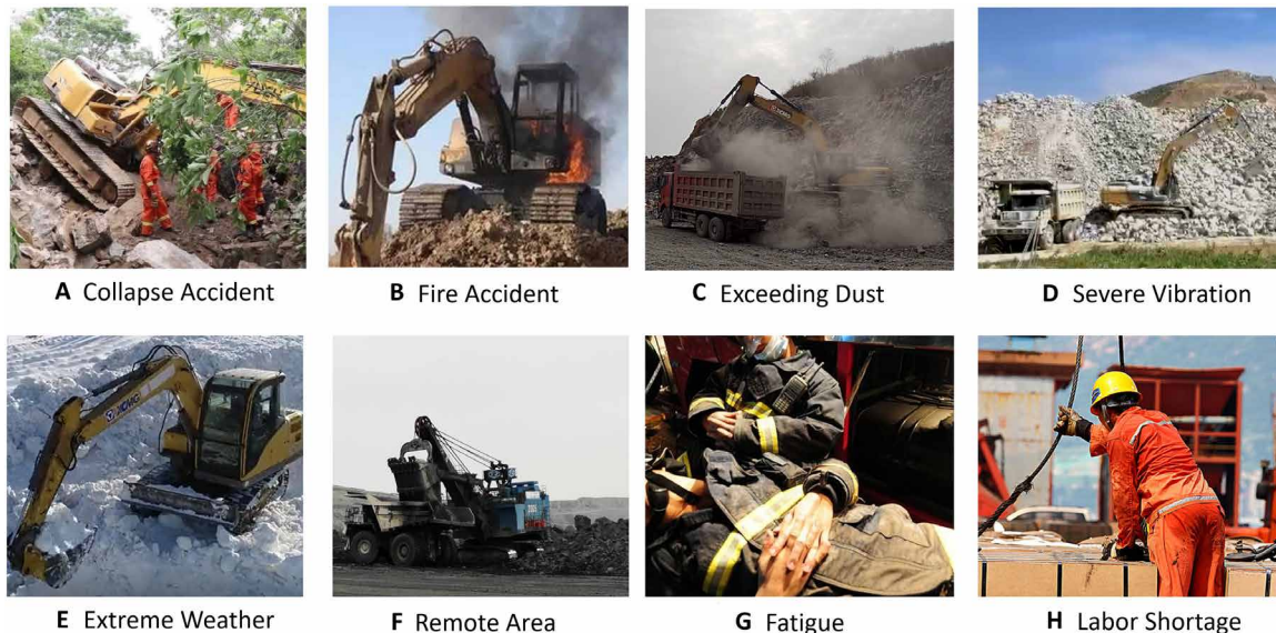
Fig. 1. Challenges with respect to using excavators. (A) Land fall in excavation sites that cause excavator accidents, resulting in casualties or injuries of human operators. (B) An excavator that caught fire in an accident. (C to F) Excavators operate in extreme working conditions, such as excessive dust, severe vibration, high and low temperatures, or in remote areas. (G) Human fatigue impairs an excavator operator's ability to safely and effectively perform the job. (H) The mining and construction workforce is facing aging issues and labor shortages in terms of operating heavy equipment, such as excavators. Our AES system is designed to address these challenges and operate automatically without any human operator intervention in challenging scenarios.
