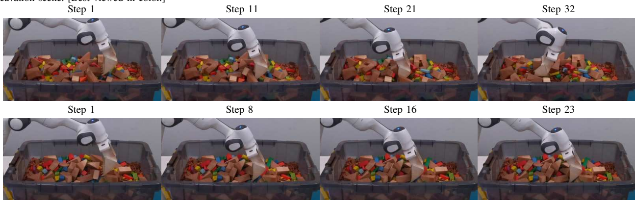
Fig. 7. The top and bottom rows show two example trajectories executed with MCTS, k = 5 , tracking the deep trajectory. In the top row, a few objects are successfully excavated, while the excavation is aborted due to large contact forces in the bottom row.
