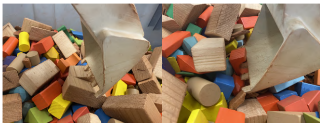
Fig. 8. Two cases that led to jamming. On the left, big blocks prevented penetration. On the right, the digging bucket teeth caught a red concave object. [Best viewed in color.]
