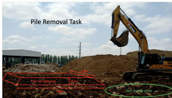
Figure 10. Pile removal experiment setup.
